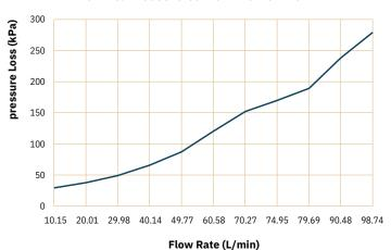
Flow vs. Pressure curve - Pump Inlet
